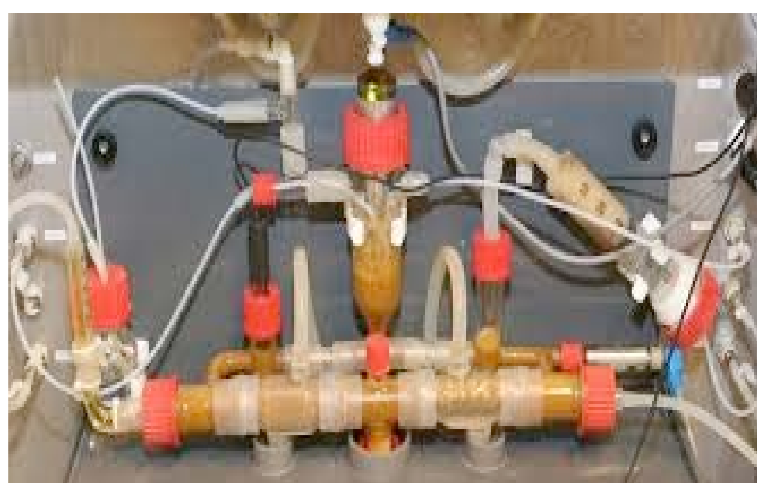
Figure 1: TIM-2, an In vitro model that mimics the conditions in the human colon
